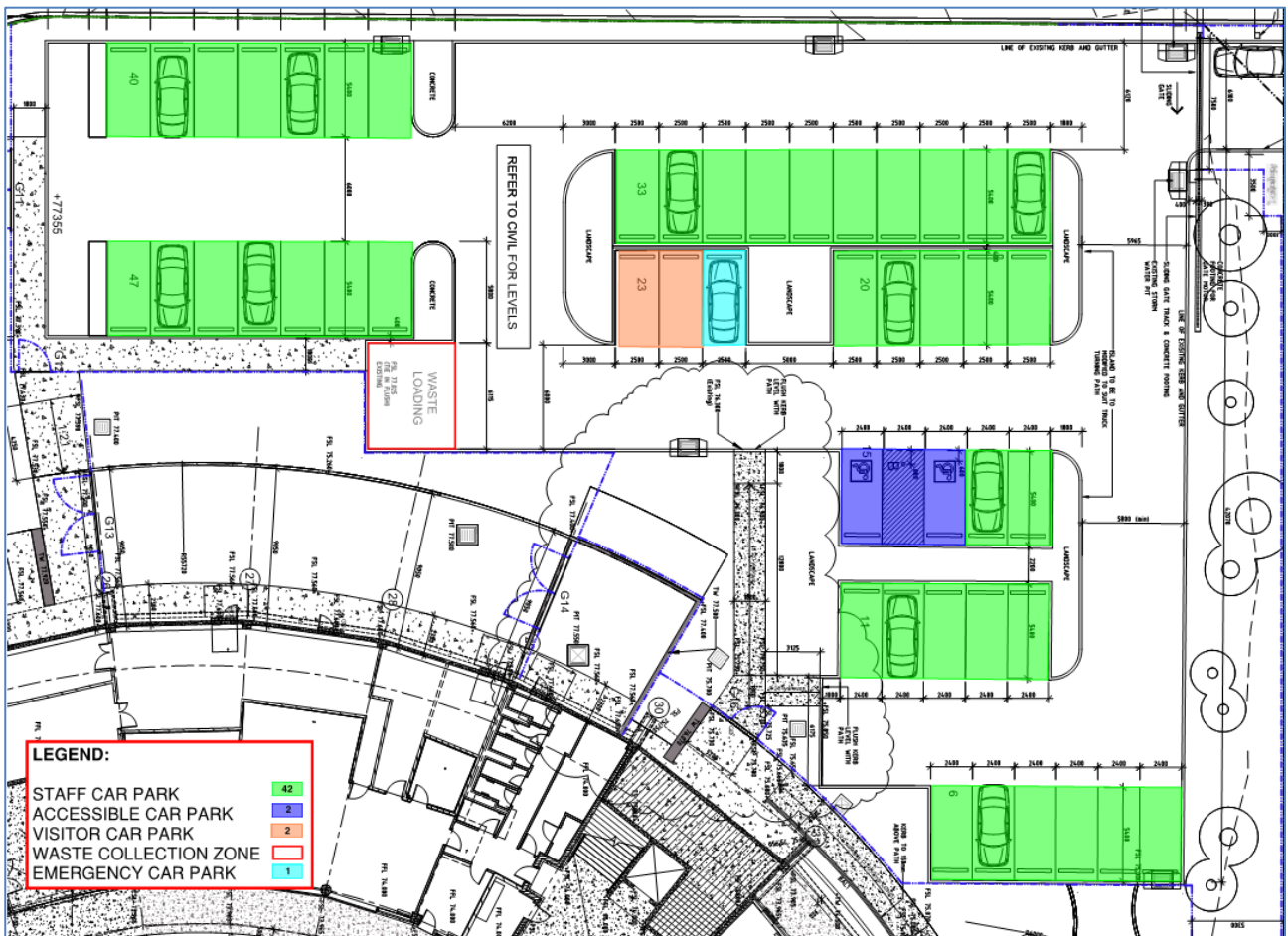
Figure 3.11: Off-street car parking allocation
